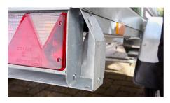
At the rear of the trailer, to the left and right of the tail lights are holes provided for the mounting of the tilt wheels.
