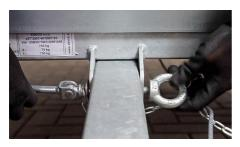
Insert the security bolt into the aligned holes and ensure the security bolt passes all the way through.
