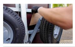
Remove the cardboard placed between the wheels and the cargo bay.
