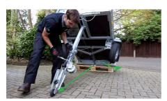
The weight of the trailer will now aid in folding out of the tow arm and under carriage (wheels & suspension). Ensure the wheels are moving into the correct load bearing position.
