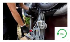
Rotate the crank handle counter clockwise for 4 revolutions to release the tension on the retractable undercarriage.
