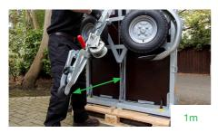
Pull the tow arm out until the undercarriage cable takes up tension.
