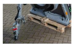
Pull the extended trailer tow arm downward so that the nosewheel touches the floor.
