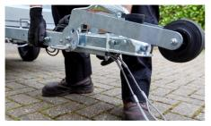
With one hand, lift the tow arm of the Foldy trailer so that the nose wheel is off the floor.
