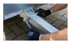
Fasten the ring nut securely with your hands to stop the security bolt from pulling out.
