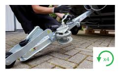
Continue turning the ratchet winch handle for an additional 4 revolution to create slack in the undercarriage cable.
