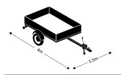
Ensure there is at least 4m by 1.5m space available from the edge of the pallet to assemble the trailer.
