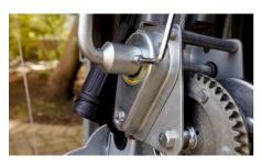
Securely fasten the two M6 Allen bolts the using the Allen key provided.
