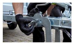
Reinsert and fasten ring nut securely in order to keep the nose wheel in place.
