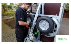
With the other hand, pull the folding tow arm out by its handle until the undercarriage cable takes up tension.
