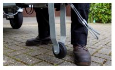
With your other hand, now rotate the nose wheel to the perpendicular position.
