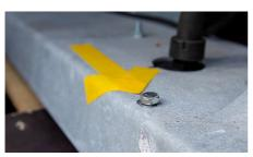
Using the size 10 box spanner provided, loosen and remove the two 120mm pallet fastening bolts at the base of the trailer.
