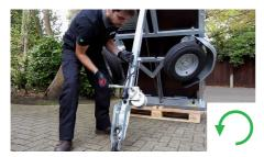
Continue to unwind the ratchet winch by rotating the crank handle counterclockwise.
