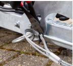
With a pair of side cutters, release any zip ties holding the electrical connector socket and the tow hinch safety cables to the tow arm.
