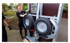
Ensure that one person continues to hold the trailer safely, while the other completes the tasks for STEP 8 through 9.
