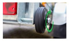
Tighten the bolt until the rotation of the wheel becomes interfered. Now loosing the bolt and nut approximately ½ a turn so that the wheel can rotate freely.
