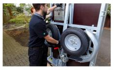
Place one hand back on the trailer to the side of folding tow arm to hold trailer stable. You might need to push the trailer slightly away from you with the hand holding the trailer. This will take the pressure off the nose wheel resting on blocks allowing the tow arm to move freely.
