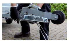
Loosen the ring nut holding the nose wheel arm in place.
