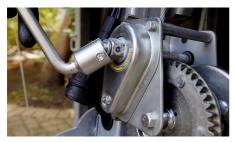
Attach the crank handle to the winch as shown.
