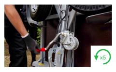
While keeping one hand holding the trailer secure, rotate the crank arm counter-clockwise an additional 5 revolutions to release further tension on the retractable under carriage.
