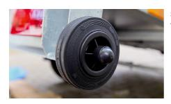
Slide the protective cap over the bolt head to complete.
