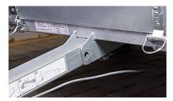
The trailer should rest with the holes for the security bolt aligned.
