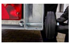
Insert the tilt wheel with the bolt head and wheel facing the outside.
