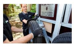
Manually pull each wheel out by about 20cm. This will free space for the folding tow arm top move out.
