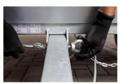
Insert the security bolt into the aligned holes and ensure the security bolt passes all the way through.
