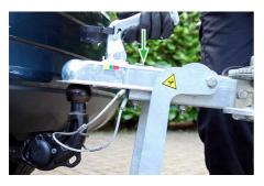
Now push down on the tow arm so that the handle forces shut as the socket-joint makes a secure coupling with the ball-joint of the tow bar.
