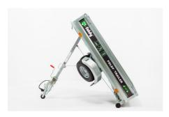
Stop rotating the crank handle when the trailer has been raised approximately 45 degrees off the floor.
