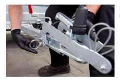
Loosen the ring nut holding the nose wheel in place.
