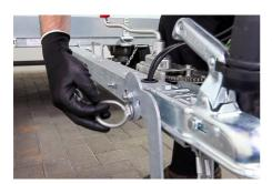
Loosen the ring bolt on the nose wheel and extend the arm forward.
