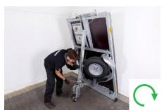
Continue to turn the crank handle raising the trailer up to the near vertical position.
