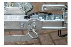
Reinsert and fasten ring nut securely in order to keep the nose wheel in place.
