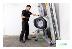
Pull the folding tow arm out by its handle until the undercarriage cable takes up tension. If the tyres interfere with the tow arm, manually pull each wheel out by about 15cm to free some space for the tow arm to move between them.
