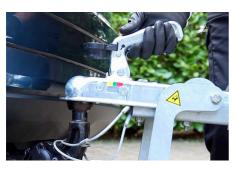
Lift the handle on the Foldy trailer's socketjoint, lowering it onto the ball of your car's tow bar.
