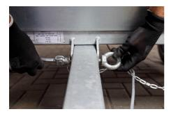
Remove the tow arm security bolt by loosening the ring nut and pulling the bolt out. You may let the securing bolt dangle temporarily by its chain.
