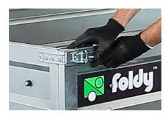
Ensure the sidewall latches of the trailer are securely closed.
