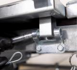
Loosen the 4 safety bolts holding front and rear sidewalls flat on the trailer deck.
