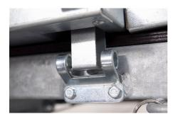
Align the hooks of the front and rear sidewalls with the hinges at the front of the trailer.
