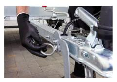
Reinsert and fasten the ring nut securely in order to keep the nose wheel in place.
