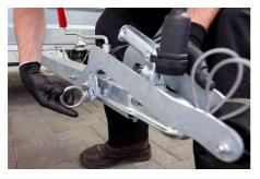
Once the nose wheel is extended, reinsert the ring bolt and fasten the nose wheel arm.
