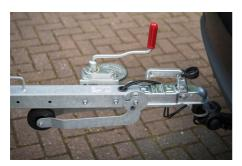
Rotate the nose wheel arm away from the car so that it is parallel to the trailer tow arm.
