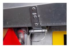
Now mount the rear sidewall (tailgate) by inserting the safety bolts into the hinges from below.
