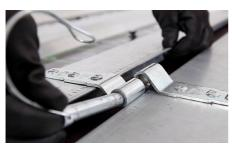
With the remaining 2 safety bolts, align the hinges of the bottom and top sidewalls and then insert them, securing the safety clips. This will ensure that sidewalls lie flat on the trailer's cargo deck.
