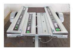
The front and rear sidewalls should both lie neatly within the left and right sidewalls.
