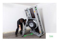
Because the trailer is in the near vertical position, you might need to assist pulling out the tow arm to about 1m from the trailer before the weight of the trailer will maintain tension on the undercarriage cable.
