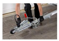
With one hand, lift the tow arm of the Foldy trailer so that the nose wheel is off the floor.
