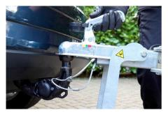
If the tow arm socket-joint does not naturally rest on the ball-joint and tips up, you must redistribute the load in the cargo bay to ensure there is enough natural downward pressure onto the tow bar.
