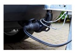
Connect the 13-pole electrical plug to its corresponding receiving socket on your car. Turn the plug connector clockwise about 45 degrees to ensure it is locked.
