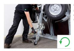
While keeping one hand holding the trailer secure, rotate the crank arm counter-clockwise to contiune releasing the undercarriage.
