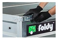
Now raise the rear sidewall and fasten the latches.
