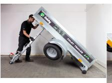
Leave about 60cm (24 inches) space between the small tilting wheels at the rear and the wall.
