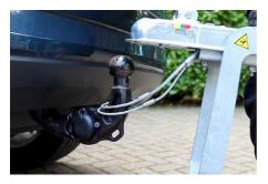
Place the safety cables over the tow bar ball-joint of your car.
