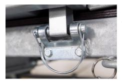
Insert 2 safety bolts through the front hinges and fasten the safety clips to hold the front and rear sidewalls in place.
