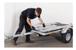
Place the front and rear sidewalls between left and right folded down sidewalls.
