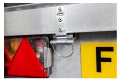
At the rear of the trailer, check that the wire clips or loops of the rear safety bolts at the tail gate are folded flat against the trailer before you start folding the trailer.
