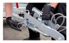
Once the nose wheel is extended, reinsert the ring bolt and fasten the nose wheel arm.
