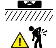
For safety reasons, ensure the folding of your trailer is completed on a flat (horizontal) and stable floor free of any debris.
