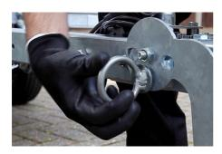
Loosen the ring nut holding the nose wheel in place.
