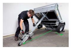
Beyond 1m, the weight of the trailer will now aid in the folding out of the tow arm and undercarriage (wheels and suspension arms).
