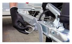
Loosen the ring bolt on the nose wheel and extend the arm forward.
