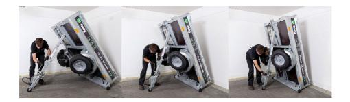
Stop rotating the crank handle when the trailer approaches the near vertical position.
