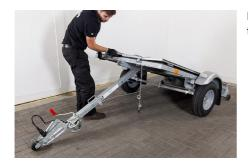
Lift the trailer to create an angle between the cargo bay and tow arm.
