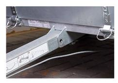
Ensure the holes for the security bolt are correctly aligned.
