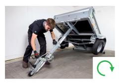
Turn the ratchet crank handle clockwise to raise the trailer off its wheels.
