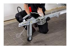
With your other hand, now rotate the nose wheel to the perpendicular position.
