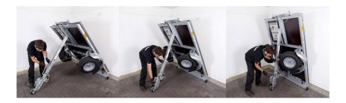
Stop rotating the crank handle when the trailer approaches the near vertical position.
