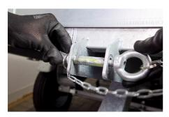
Reinsert the security bolt back through the holes on the cargo bay bracket and thread the ring nut partially (3 turns) to hold the bolt in place.
