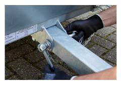
Fasten the ring nut securely with your hands to stop the security bolt from pulling out.
