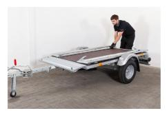
Unlatch all the sidewalls and fold the left and right sidewalls down so that they are lying flat on the cargo bay deck.
