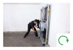
Turn the ratchet crank handle until the tow arm is in the fully closed position.
