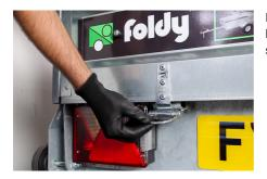
Remove the front and rear sidewalls by pulling the safety bolts out from the sidewall hinges.
