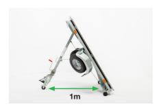
THE TOW ARM MUST EXTEND AT LEAST 1 METER FROM THE TRAILER WHEN MOVING.
